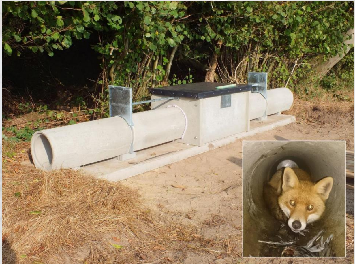
Automatic live trap with mobile sensor
